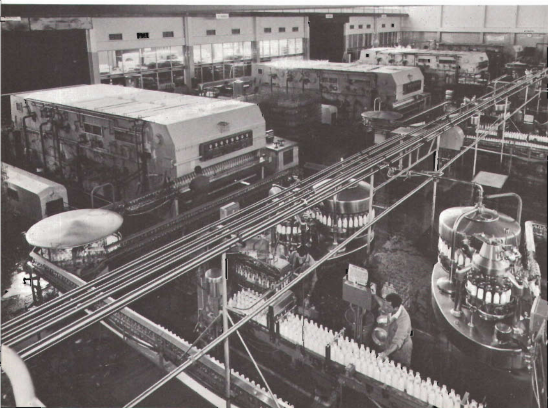
A view of modern machinery used for automatic washing, sterilising, and milk filling in a Broadmeadows plant. [Metropolitan Dairies
